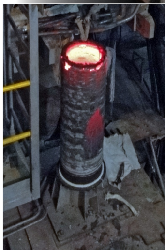
Smelting of hollow billet using the furnace ESRF-15/30.
