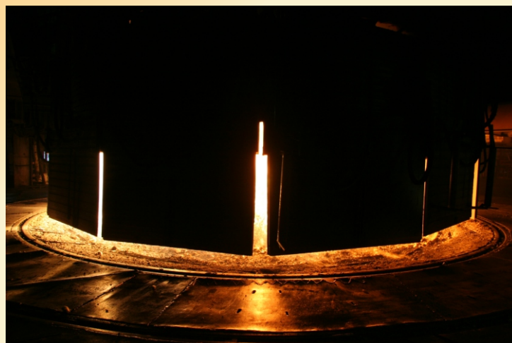
RKO-25 ore thermal furnace (capacity: 25 MVA) for production of high-grade ferrosilicium and silicon (construction of VNIIE TO)
